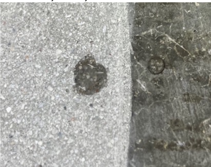
Figure 11 - Check for absorbency using methods outlined in ASTM F3191
