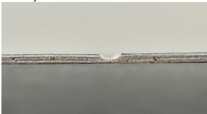
Figure 19 - Grooves shall be cut to a depth equal to two-thirds (66%) of the product's total
