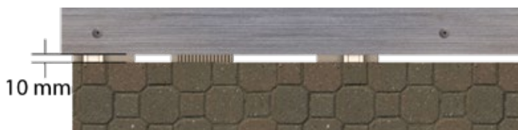
62. Minimum distance between the moulding and floor.
