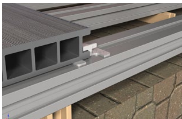
41 Clip and stainless steel screw on an aluminium batten. Deck header resting on the batten.
