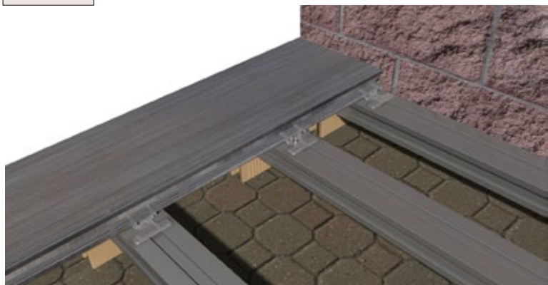
39. Fastening the deck with Tarimatec® clips
