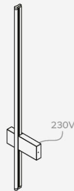
230V gearbox with integrated 24Vdc power supply can be placed anywhere along the profile.
