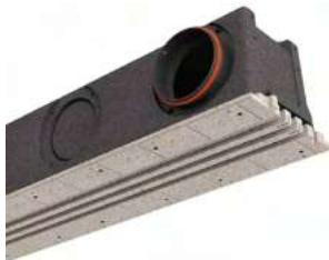
**LINEO PRO CONDI** is designed for duct systems with diameters of 150 mm and 160 mm. The three diffuser slots are designed to allow for the extremely high air flows typical of cooling systems.
