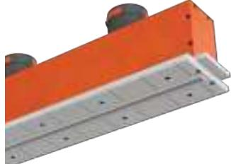
**PROFILE 600 VERTICAL** model diffuser is specifically designed for installation on the "face" of the plasterboard ceiling. It connects to a flexible 75 mm plastic duct system and requires only 17 cm of space for installation.
