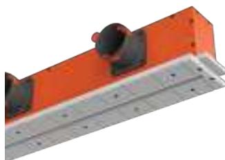
**PROFILE 600** model diffuser is designed for plasterboard ceilings / walls, connecting to a 75 mm flexible duct system. The design is compact, requiring just 17 cm of installation depth.
