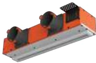
**SINGLE 500** model diffuser is designed for plasterboard ceilings / walls, connecting to a 75 mm flexible duct system, contains a balancing valve & **needs only 12 cm for installation.**
