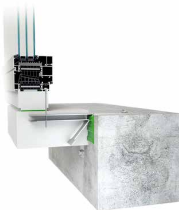
Bottom connection, 200 mm beam with internal anchor
