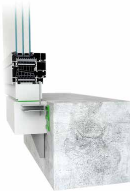
Bottom connection, 100 mm beam with external anchor
