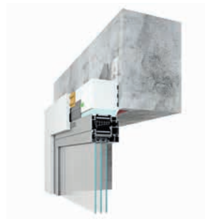
top connection, with jamb external profile
