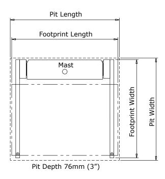
If a pit is used, recommended depth is 76mm (3"). Pit width and length include running clearances.
