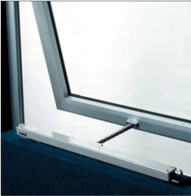
SYNCHRO QUASAR DC DRAWBRIDGE Installation on bottom hinged window, opening outwards 90°: The actuators are equipped with a special guide for the chain. Contact our Technical Department for the installation limits (size and weight of window) and brackets for actuator installation (depending on type of profile)
