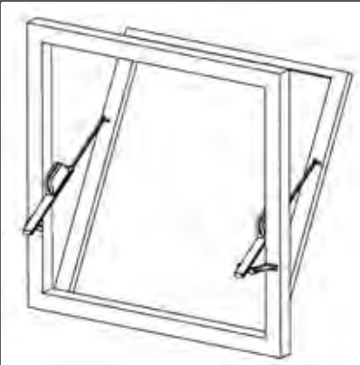
Installation on bottom hinged windows outward opening
