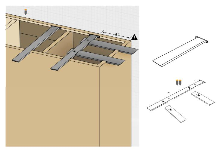
**1.** Measure and mark the appropriate mounting locations on the inside face frame or front gusset and corresponding position on the back edge of the cabinet. We recommend starting the brackets 6" in from the edge of the cabinet.
