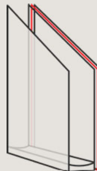
Laminated safety glass (LSG) with single or double PVB film
