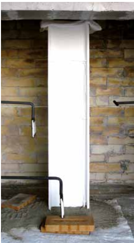
Steel beam with C-THERM® before the fire test.
