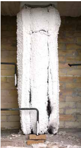
Steel beam with C-THERM® after the fire test.
