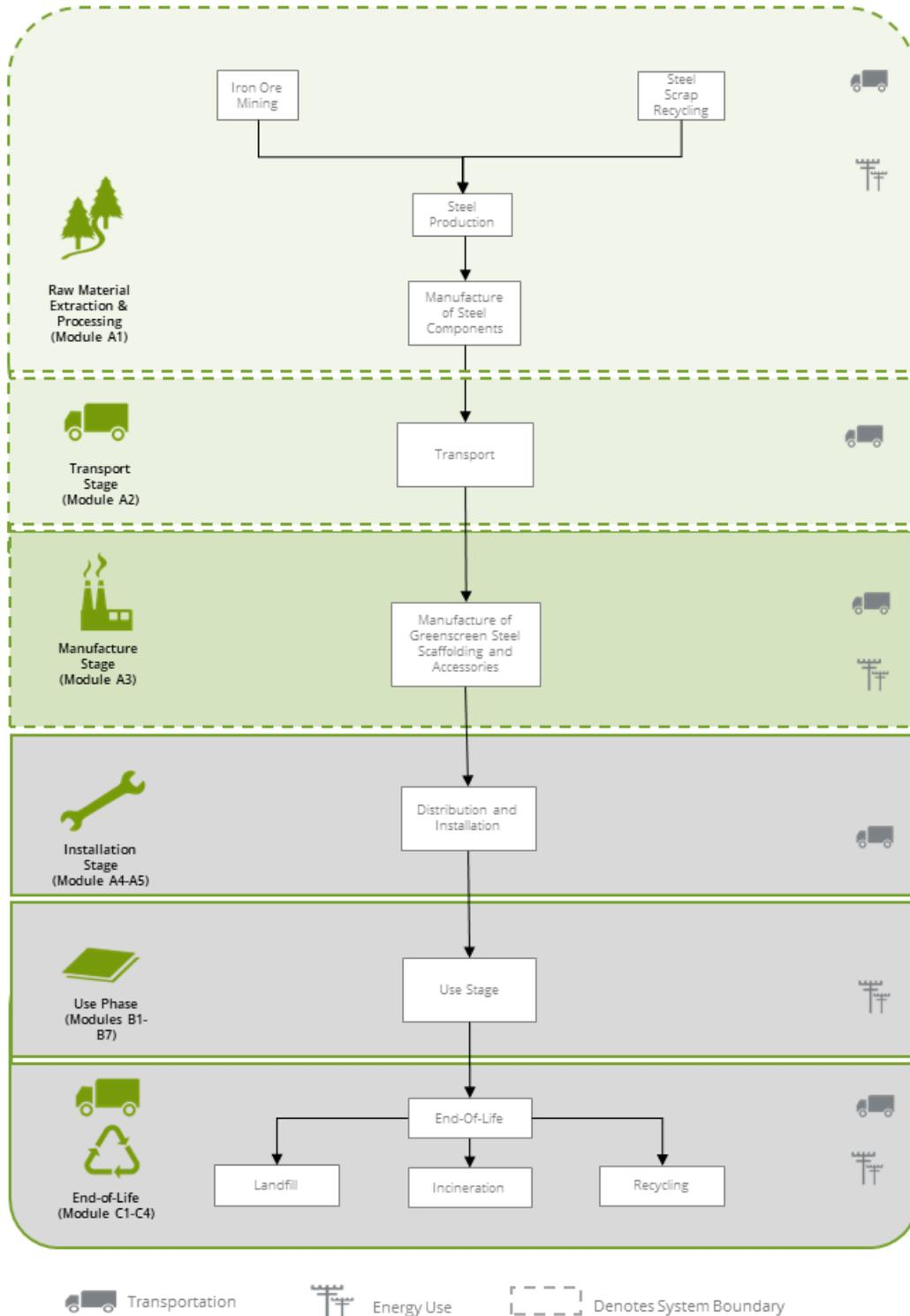
Figure 1. Flow Diagram for the life cycle of the Greenscreen welded wire trellis system.
