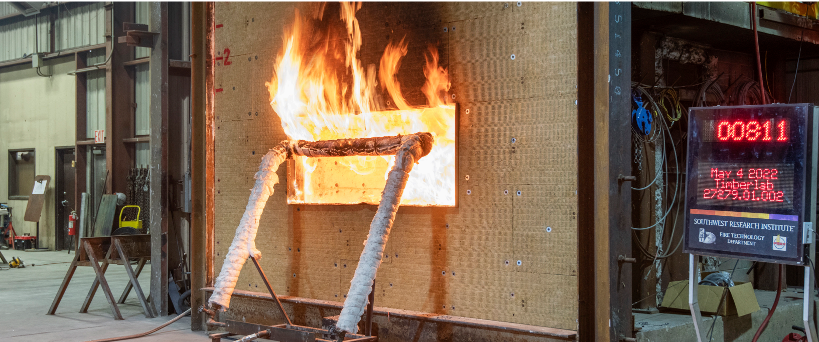
The two-story testing wall exposed to flaming at temperatures over 1600 °F. Courtesy photo by Erika Edwards.
