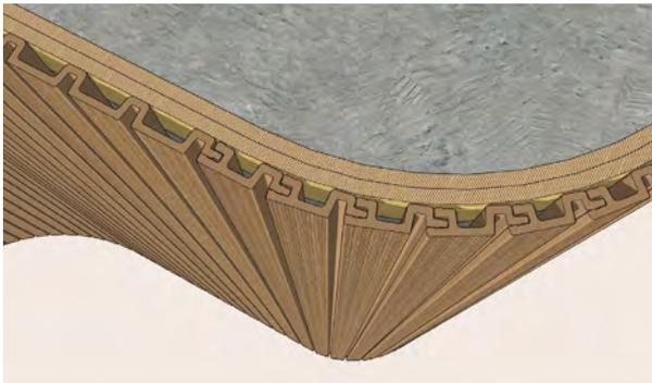
Vertical installation on convex curved wall with a minimum radius of 1m
