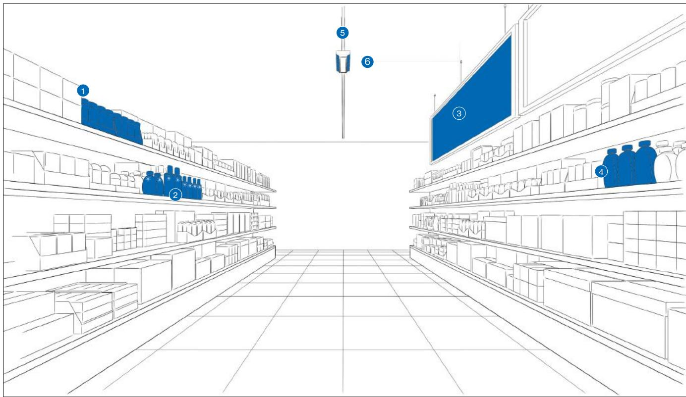
**EN** SQUADRO combines all the advantages of traditional retail lighting solutions in one luminaire. The spotlights are transversely and longitudinally glare-free and direct the light precisely onto the goods – into the heights and depths of the shelves. This achieves a strong product presentation. Thanks to proper light distribution, no additional light source is required for basic lighting.
