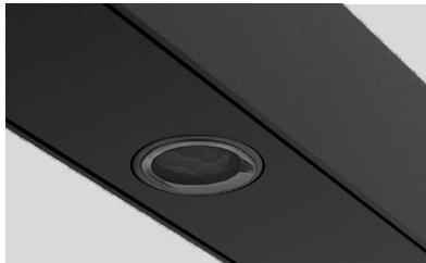
**EN** BETO System is equipped with a DALI sensor and can be controlled as a network. A presence sensor controls the light at the workstation if someone is there. A brightness sensor adjusts the light intensity to the ambient brightness. If desks, rooms, or corridors are unoccupied, the light automatically switches off after a defined delay. This saves energy and extends the service life.
