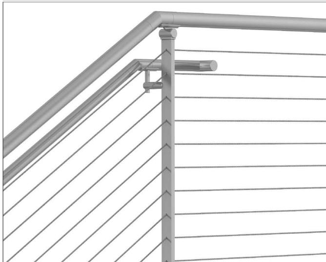
VIVA's stainless steel cable infill is a low maintenance, high visibility infill that is popularly used on exterior applications. Our cable comes in 1x19 type weave, 3/16" diameter in SS316 alloy.
