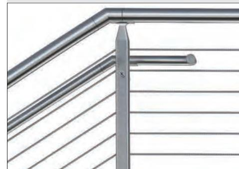
VIVA's stainless steel cable infill is a low maintenance, high visibility infill that is popularly used on exterior applications. Our cable comes in 1x19 type weave, 3/16" diameter in SS316 alloy.
