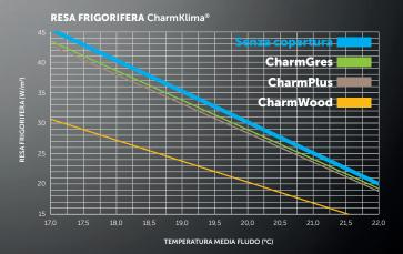
For panels with a 28 mm gypsum fibreboard core, the delivery temperatures shown in the table must be increased by 7%.
