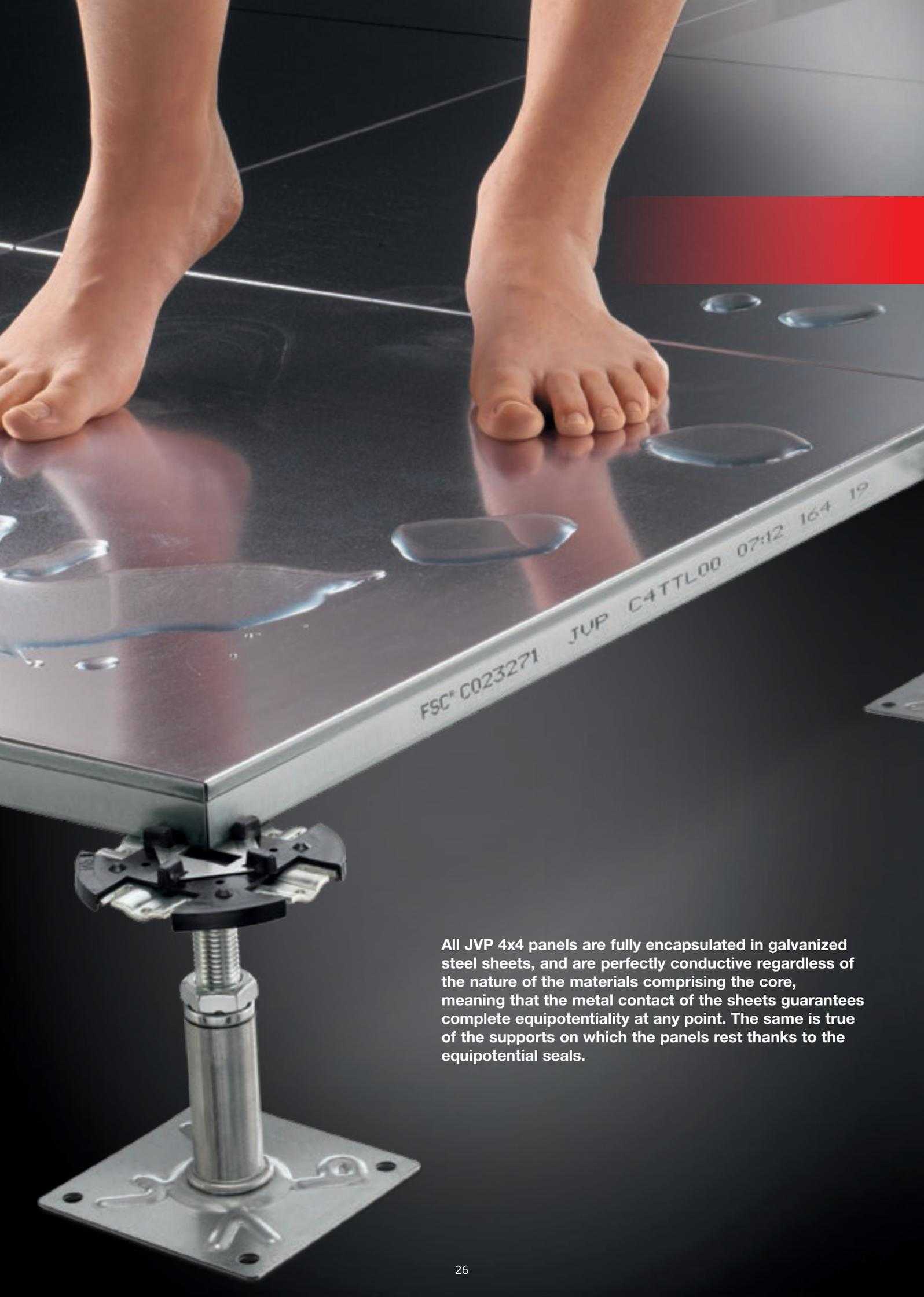
All JVP 4x4 panels are fully encapsulated in galvanized steel sheets, and are perfectly conductive regardless of the nature of the materials comprising the core, meaning that the metal contact of the sheets guarantees complete equipotentiality at any point. The same is true of the supports on which the panels rest thanks to the equipotential seals.
