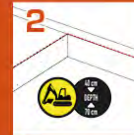
Prepare the ground.
