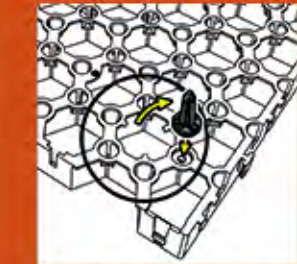
When laying on a slope, please cut and use the anchoring pins, and insert them into the underside of the tile for extra grip.
