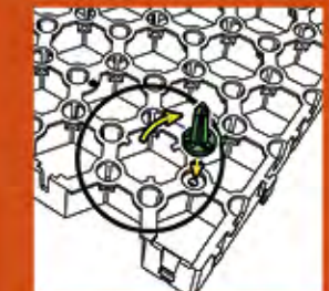
Insert them into the underside of the tile for extra grip.
