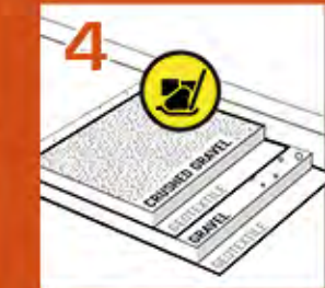
Lay the draining and the upper sub-base.
