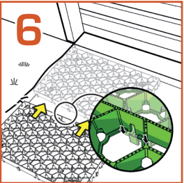
Pose de Greenplac®.
