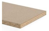
Wood particleboard Type P5 in accordance with EN 312, for load-bearing boards for use in humid conditions and with increased water vapour diffusion resistance.
