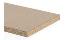
Urea resin-bonded particleboard, type P2 conforming to EN 312, suitable for non load-bearing purposes in dry areas.
