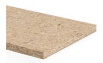
Wood particleboard type P5 in accordance with EN 312, for structural purposes, for use in humid conditions, uncoated and 100 % formaldehyde-free bonding.
