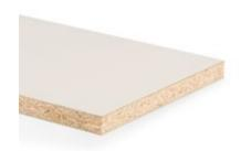
Wood particleboard type P6 in accordance with EN 312, heavy-duty, for structural purposes for use in dry conditions, melamine faced on both sides, flame retardant.
