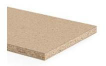
Wood particleboard type P7 in accordance with EN 312, heavy-duty, for structural purposes for use in humid conditions, unfaced and 100 % formaldehyde-free bonding.
