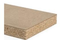
Wood particleboard type P6 in accordance with EN 312, heavy-duty, for structural purposes for use in dry conditions.
