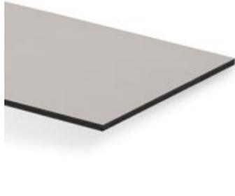
Compact high-pressure laminate for outdoor use in flame retardant quality according to EN 438-6:EDF / intensive decors according to EN 438-6:EGF. With uniform black-coloured core and single-sided decorative acrylic lacquer on the top side and decorative melamine resin surface on the reverse.
