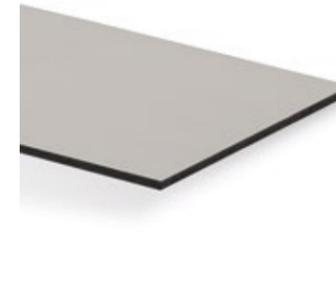
Compact high-pressure laminate for outdoor use in standard quality according to EN 438-6:EDS / intensive decors according to EN 438-6:EGS. With uniform black-coloured core and single-sided decorative acrylic lacquer on the top side and decorative melamine resin surface on the reverse or double-sided decorative acrylic lacquer.
