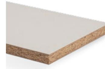
Combination of particleboard (MFP) as middle layer and one high-density thin fibreboard (HDF) as top layer on each side with decorative melamine resin facing on both sides.
