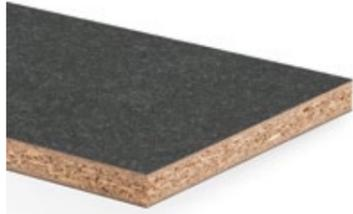
HPL bonded board consisting of a particleboard type P2 to EN 312, surfaced on both sides with Duropol XTreme Touch, an attractive supermatt surface material with an anti-fingerprint effect in combination with natural-looking stone or wood structure.
