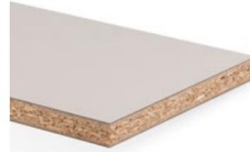
HPL bonded board consisting of a particleboard type P2 to EN 312, surfaced on both sides with Duropol XTreme plus, an attractive supermatt surface material with an anti-fingerprint effect, which is ideal for horizontal, heavily used surfaces.
