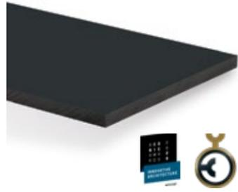
Compact high-pressure laminate in standard quality in accordance with EN 438-4:CGS or EN 438-9:BCS. With uniform black-, grey- or white- coloured core and electron beam cured surface on both sides. Duropol Compact XTreme plus is an attractive supermatt compact material with an anti-fingerprint effect, which is ideal for horizontal, heavily used surfaces.
