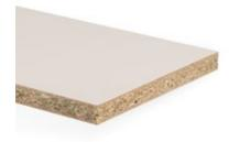
Wood particleboard type P7 in accordance with EN 312, heavy-duty, for structural purposes, for use in humid conditions, melamine faced on both sides.
