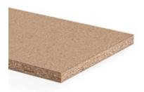
Wood particleboard type P7 in accordance with EN 312, heavy-duty, for structural purposes for use in humid conditions, unfaced and 100 % formaldehyde-free bonding.
