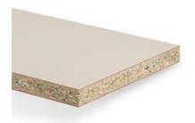
Flat bonded element consisting of a moisture-resistant particleboard type P3 to EN 312 for damp areas, surfaced on both sides with Duropal HPL.
