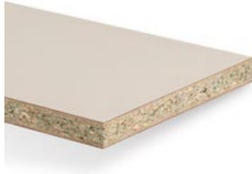
Flat bonded element consisting of a moisture-resistant particleboard type P3 to EN 312 for damp areas, surfaced on both sides with Duropol HPL.
