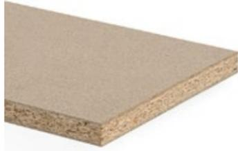
Chipboard bonded with 100 % biogenic, formaldehyde-free glue (OrganicGlue) with a recycled wood content of approx. 100 % type P2 according to EN 312, suitable for non-load-bearing purposes in dry areas.
