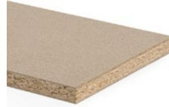
Chipboard uniformly bonded with biogenic, formaldehyde-free glue (OrganicGlue) with a recycled wood content of approx. 50 % type P2 according to EN 312, suitable for non-load-bearing purposes in dry areas.
