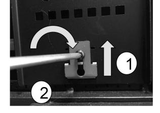
Align tray mounting clips and center mounting bracket into top and bottom cabinet rails. Orient the rails so that center mounting bracket points down and the PDU mounting keyholes (if present) are properly oriented
