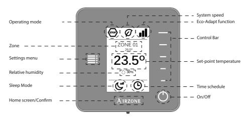
**Operating modes:** It displays the operating mode selected from the Master controller (or from the Think thermostat if configured as Master). These are 5 available modes: cooling, heating, dry, ventilation and stop (see *settings menu* on page 16).
