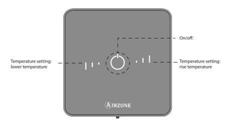
**On/off:** On/off of the zone. In addition, it indicates the operating mode by using different colours. (see *On/off* on page 19).
