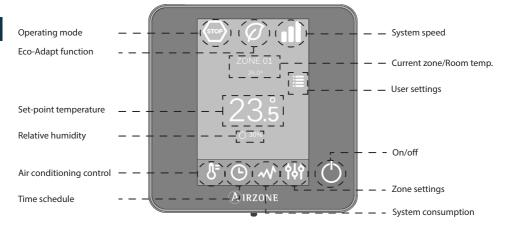
**Operating modes:** Select among the available modes: cooling, heating, dry, ventilation and stop. (See *air conditioning control and operating modes on* pages 6 and 7).
