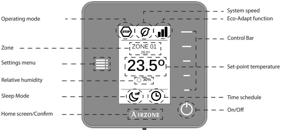
**Operating modes:** It displays the operating mode selected from the Master controller (or from the Think thermostat if configured as Master). These are 5 available modes: cooling, heating, dry, ventilation and stop (see *settings menu* on page 16).
