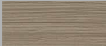
130/11 - Boxwood Topped with Scumble Driftwood
