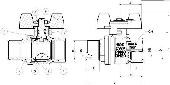
DN shows the nominal flow diameter. Actual flow diameter complies with full port DIN 3357 part 4.
