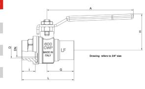
DN shows the nominal flow diameter. Actual flow diameter complies with full port DIN 3357 part 4.
