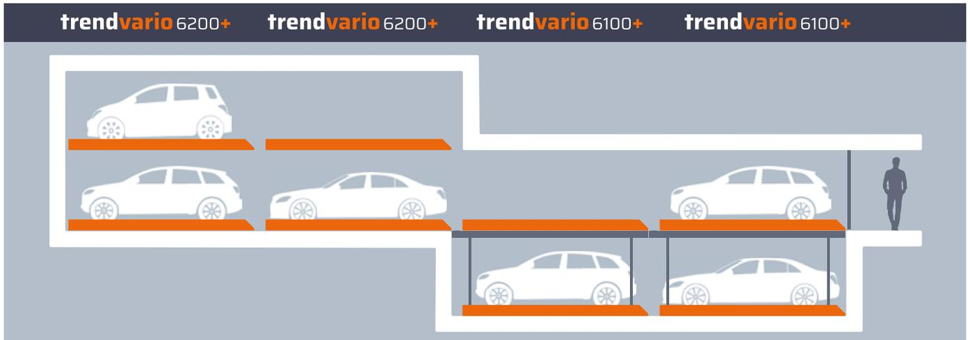
All TrendVario+ models can be combined any way you like, one after the other, in up to four rows. The “plus” stands for the model that can be driven on.
