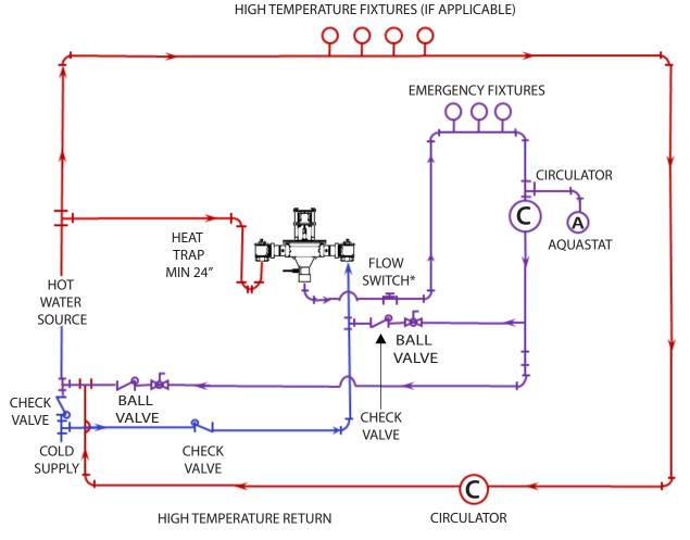
\*FLOW SWITCH MUST BE LEVEL AND IN CORRECT DIRECTION
