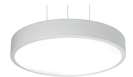
RNDP | Round Architectural Pendant Featuring 2' & 3', 1,800 - 5,200 lumens, 80 CRI, 4000K CCT, frosted convex acrylic lens, pendant mount, white finish
