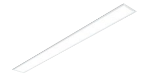
MX4R | 4" Continuous – Recessed Featuring 4' & 12', 800 lumens per foot, 80 CRI, 4000K CCT, flat diffuse acrylic lens
