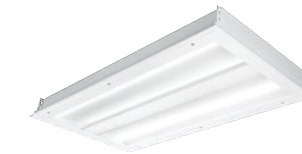
MCTM | Multi-Function Medical Featuring ambient, exam, reading & night styles, 4,700 ambient & 8,400 exam lumens, 80 CRI, 4000K CCT, straight diffuse acrylic insert with polycarbonate underlay
