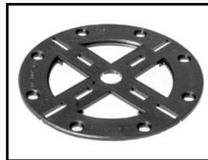
Uni-Shim™ 1/8" and 1/16": Allow for fine tuning of individual pavers. Can be broken into quarters or halves and stacked on top or bottom of pedestals.
