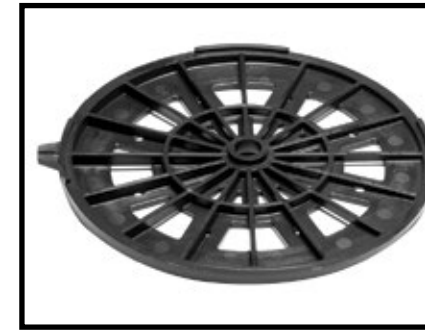
Base Slope Plate: Used for slope compensation at base of pedestals. Each plate compensates for 1/4" per foot (2%) slope and adds 3/8" to the overall height of pedestal. Maximum of four plates may be stacked for compensation of up to 1" per foot (0-8%) slope.
