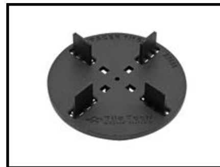
Spacer 1/16" (2mm): Used with Hex and Turf-Trays. Allows for 1/16" spacing gap between pavers for drainage. Tabs are perforated for easy removal.
