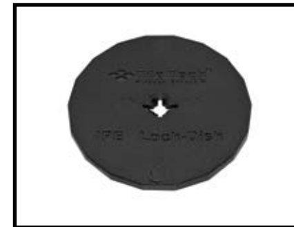
IPÉ Lock Disk: Used to secure wood tiles by inserting disk into kerf-cut between the upper slat and bottom rail, adding the 4th tile and securing with 1-1/4" deck screw.
