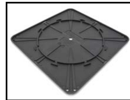
Foundation Pad: Used under pedestals for on-grade applications. Provides a 10" x 10" larger load bearing surface area to protect base from sinking into compact gravel base.
