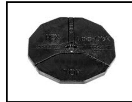
Hex-Lock Disk: Used to secure Hex-Trays to prevent wind uplift by inserting disk into kerf-cut and then securing with 1-1/4" deck screw.
