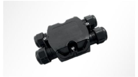
Electrical connection with quick disconnect connector in PA66 without halogens and phosphorus with silver-plated copper contacts, for cables  $\varnothing$  9 -  $\varnothing$  14 mm.
