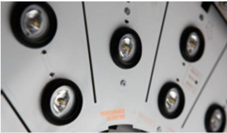
Each LED is coupled with an electronic safety device (NUD) that can by-pass it in case of failure
