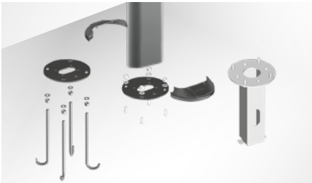
Installation can make use of the accessory stainless steel ground plate to anchor the device to cement
