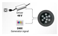
The RGBW versions should be powered at 48Vdc with SELV drivers, available as accessories. Colour management is through DMX interface.
