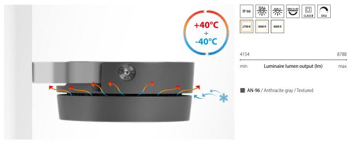
Luminaire designed with two separate die-cast aluminium compartments to maximise heat dissipation between electronic components and the LEDs, powder-polyester coated ISO 9227
