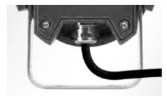
Tear-proof nickelled brass cable gland M16x1.5 for cables  $\emptyset$  5 mm-  $\emptyset$  10 mm
