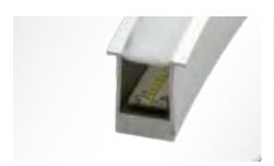
IP-67-rated double resin coating - transparent in the lower part to protect the LED from mechanical stresses and to guarantee maximum luminous efficiency - satin finish in the visible part, even in joints proximity, to ensure a homogeneous light distribution over the entire emitting area
