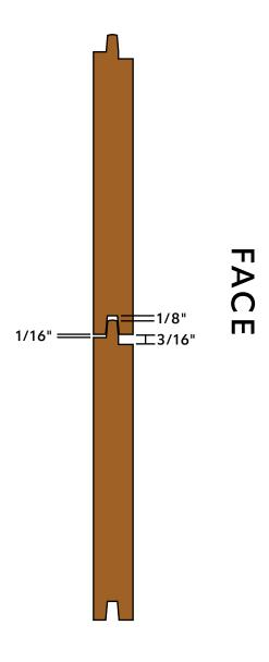
A 3/16" reveal gap should be provided between each board to allow for proper expansion and contraction during acclimation. Do not use a mallet or hammer to force boards into place
