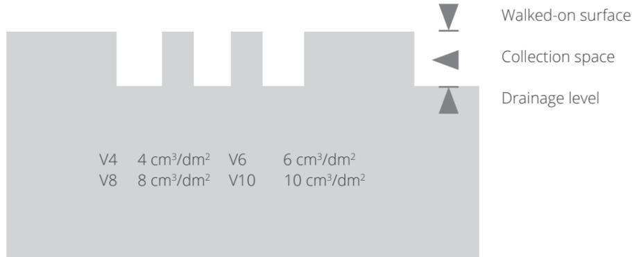
The displacement space (V4-V10) is the open space between the upper walked-on surface and the drainage level of profiled surfaces.
