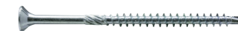
Wood drilling screw, countersunk head milling ribs, TX®, part thread, drill-tip, steel zinc plated
