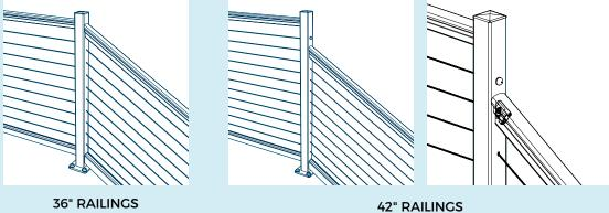
Terminate the top two Cable Runs because of the change in height.
