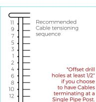
Cables can either terminate or run through Corner Posts. **DOUBLE PIPE** ANGLE IRON
