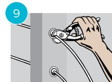
Use Cable cutters or Electric Grinder with Cut-off Disc to trim the excess Cable. Grind flush the exposed Cable ends with an Electric Grinder.
