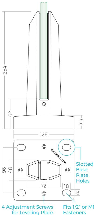
4 Adjustment Screws for Leveling Plate
