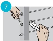
Tension the Cables by holding the Threaded Terminal shaft with Vise-Grip Pliers and spinning the Snug-Grip® Washer-Nuts with a Wrench. A Feeney Tension Gauge may be used to check uniform tension.
