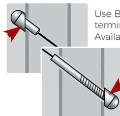
Use Beveled Washers for Stair termination Posts with angled holes. Available for both Threaded Terminal & Quick-Connect® Fittings. Always install the Quick-Connect® Fitting in top Stair Post to prevent rain water from running down the Cable into the Fitting.
