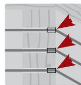
Protector Sleeves prevent abrasion at angled transitions on Wood Posts (e.g., Stair transition Posts or outside faces of Double Corner Posts). Fits 1/4" diameter drill holes.
