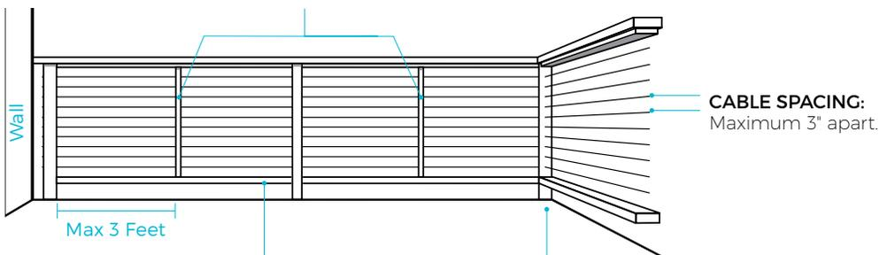
**FOOT RAILS (Optional):** Recommend minimum 2 x 4 size Wood spaced no more than 4" (or as per code) above the deck surface.
