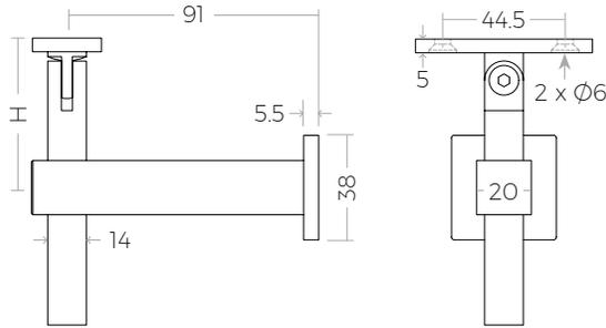
Installed with M8 Hanger Bolt
