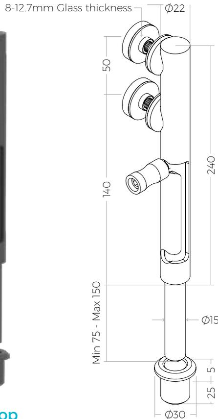
\*Floor Flange secured by #14 Flat Head Screw (not included).
