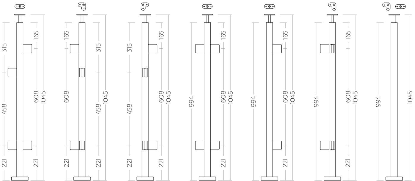
6. Transition 36/42 SSPEXS36T42    7. Transition Left SSPEXS36TL    8. Transition Right SSPEXS36TR    9. Landing Line SSPEXS42LNL    10. Landing End SSPEXS42LNE    11. Landing Corner SSPEXS42LNC    12. Blank Post SSPEXS42BL
