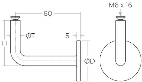
Installed with M10 Hanger Bolt
