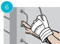
Hold the Quick-Connect®SS Fitting with one hand and pull the Cable tight with the other. The Fitting automatically locks when you release the Cable.
