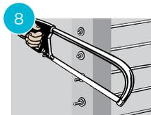
Use Hacksaw, Reciprocating Saw, or Electric Grinder with Cut-off Disc to saw off the excess threads as close to the Snug-Grip® Washer-Nut as possible. Touch up with Electric Grinder. The special Snug-Grip® threads prevent the Nut from loosening.
