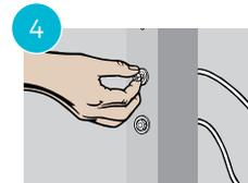
Insert the Threaded Terminal through the Terminal End Post and attach a Flat Washer and Snug-Grip® Washer-Nut. Spin the Nut 2 full turns. Strong resistance will be felt as the Snug-Grip® threads engage, so hold the Terminal shaft with pliers.
