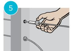
Lace the free end of the Cable through the Intermediate Posts and Quick-Connect® End Post. Slide on a Flat Washer and Quick-Connect® Fitting until they rest against the face of the Post. Use a Lacing Needle if snagging becomes a problem.
