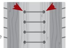
Cables can either terminate or run through Corner Posts.
