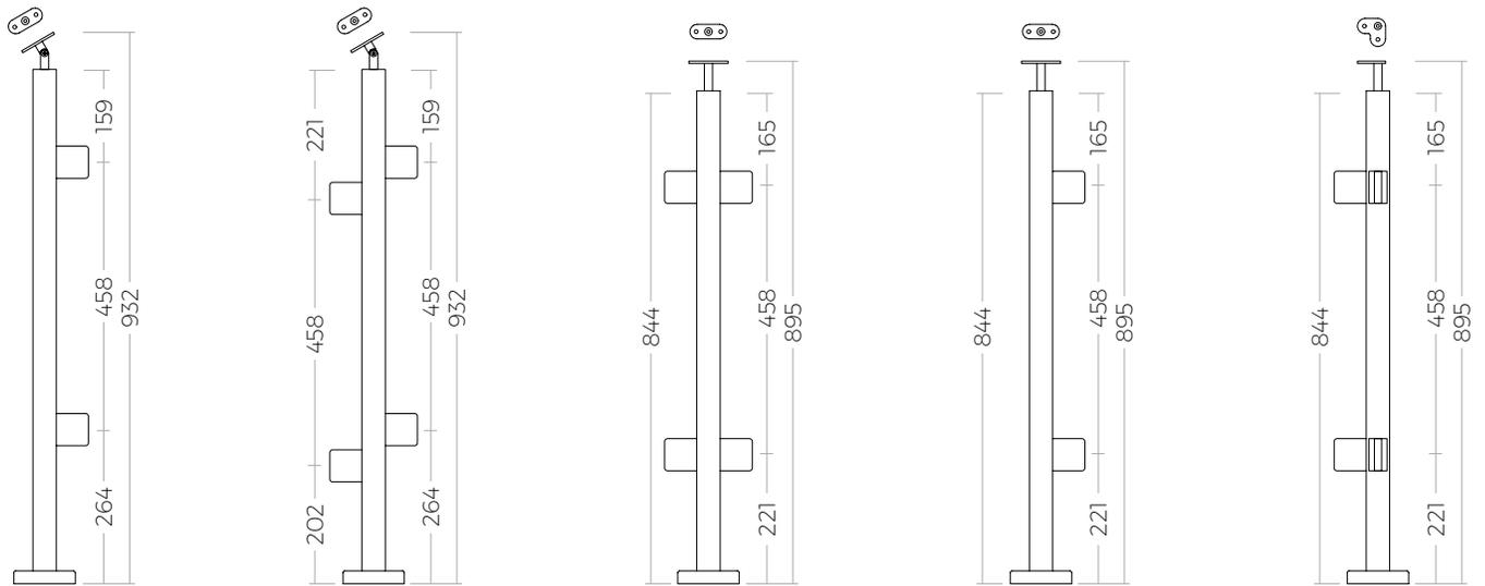
Typical Stair Configurations for 36" - 42" Posts
