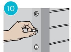
Snap on End Caps over the exposed Quick-Connect®SS Fittings and the Snug-Grip® Washer-Nuts. You're done.
