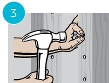
Insert Protector Sleeves at necessary locations. Tap in until flush.
