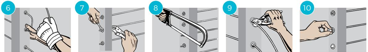
**6** Hold the Quick-Connect®SS Fitting with one hand and pull the Cable tight with the other. The Fitting automatically locks when you release the Cable.
