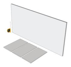
Mark out Several reference markers showing the final panel alignment should be placed on the wall.
