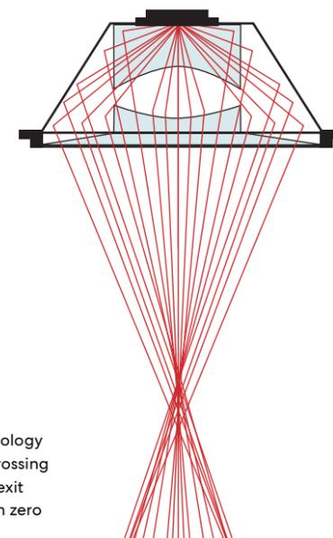
XPoint™ technology enables crisscrossing light paths to exit the fixture with zero light spill.
