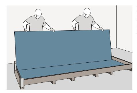
Given their reduced thickness, we suggest that the slabs always be moved by two operatives, distributing the gripping points and avoiding pressure being applied at single points when lifting the packages, as this could lead to product breakage.
