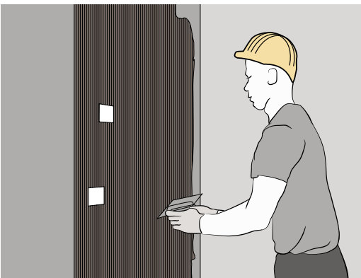
Spread adhesive on plaster
