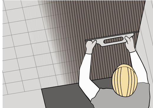
Spread adhesive on the existing substrate
