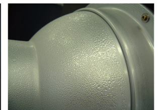
■ SpotDiffuser WITHOUT Condensation Control Air Guide
